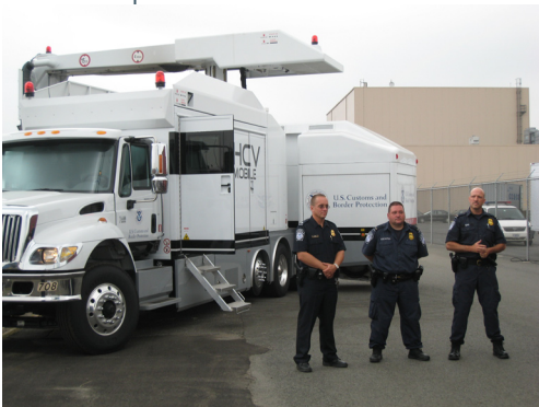
U.S. Customs HCV Mobile Cargo Screening Unit
